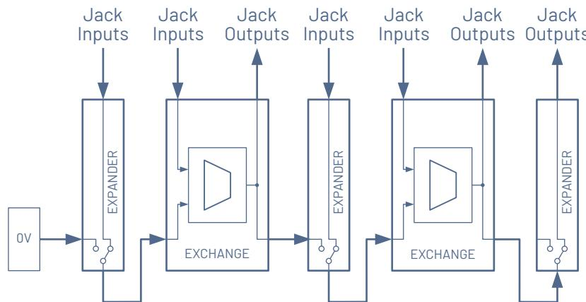
For the middle Expander, the left Exchange is normally connected to the right Exchange for each of the 8 jack sockets on the Expander where a jack is not inserted. When a jack is inserted, the chain is broken, and the right Exchange will receive the input from the middle Expander. Because the chain outputs of Exchange are buffered, any number of Exchange chain stages connected this way is possible.
