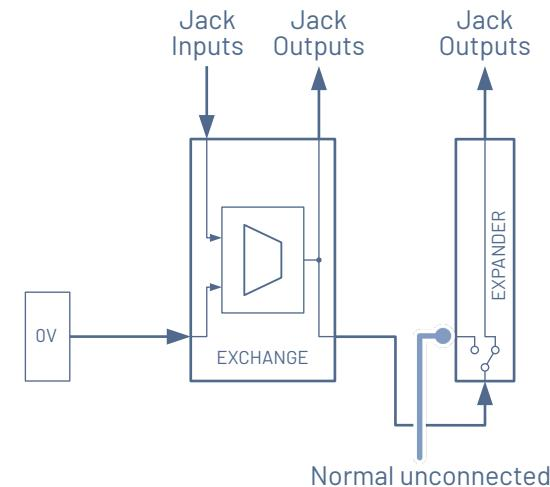
With this configuration, the jack outputs of Exchange are duplicated to the jack outputs of Expander. The jack outputs and chain outputs of Exchange are independently buffered, so the loading on one output bank by connected modules will not affect the other.
