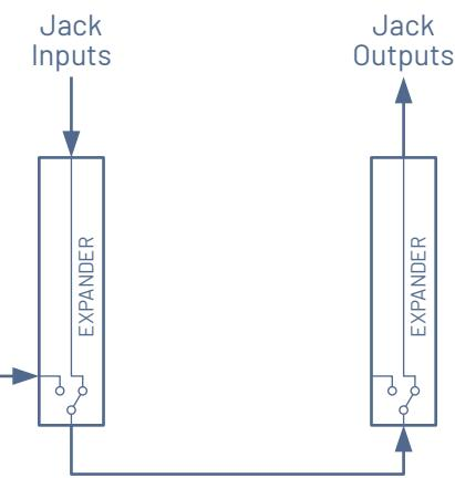
The figure below shows how the normal connections can be used to chain multiple Expanders together. The normal connected Expanders provide multiple points in the chain which can be broken by inserting a jack. The rightmost jack in the input Expanders in the chain will drive the outputs of the output Expander.
