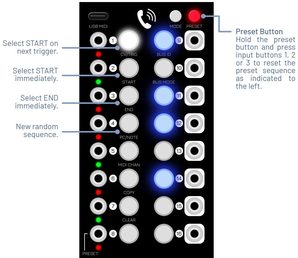
The sequence reset functions will have no effect in the preset input CV mode. The behaviour is the same for random sequences, except the random sequence will continue with a random preset on the next trigger after the reset function has completed. While PRESET is held down, buttons can be pressed multiple times to reset a sequence during a live performance.
