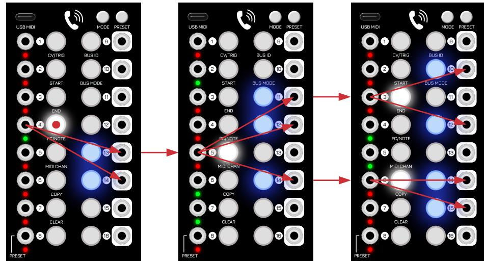
The same patch chain is shown below, except now, input 3 is held down on the right Exchange. Only outputs 10 and 12 will be highlighted this time as input 3 is now the start point of the highlighting trace. This input is then traced back through the chain to a single source.
