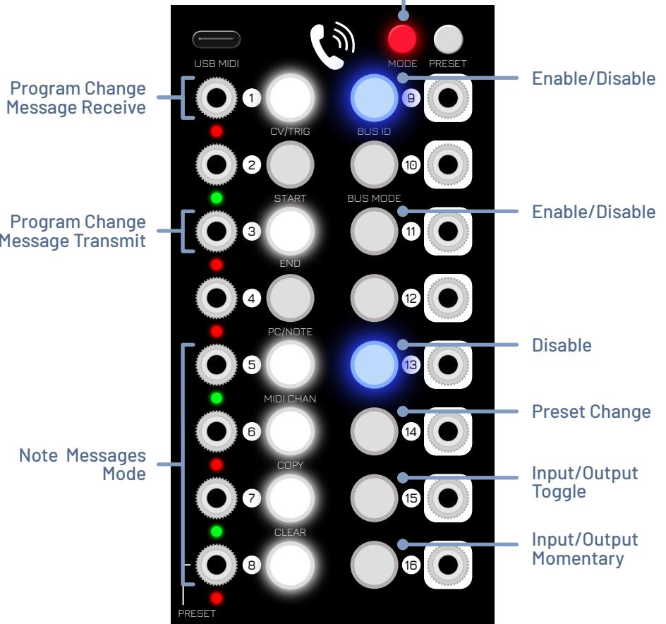
The program change (PC) message receive mode enables Exchange to load a preset in response to a MIDI PC message received from the USB MIDI port. Program change messages 0-63 correspond to presets 1-64. The enable state is indicated by the righthand button, where glowing blue indicates enabled and not glowing disabled.
